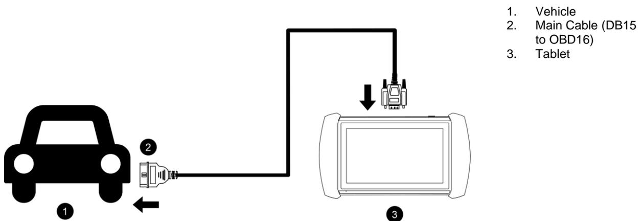
***⚠ Note: Please make sure all the cables are connected tightly; The vehicle's DLC is not always located under the dash; for the location of the DLC, please refer to the vehicle's user manual.***
