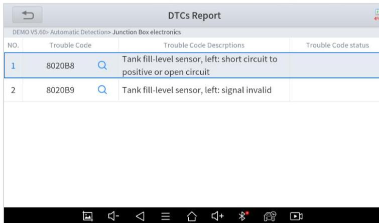
In the process of diagnosis, if the device shows “System is OK” or “No Trouble Code”, it means there is no related trouble code stored in ECU or some troubles are not under the control of ECU. Most troubles are mechanical system troubles or executive circuit troubles. It is also possible that the signal of a sensor may be inaccurate but within limits, which can be examined using Live Data.
