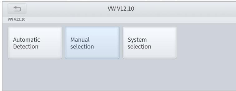
**Automatic Detection** will automatically identify the vehicle's VIN code, and then read the information of your target diagnostic object. If you choose "**Manual selection**", then you can continue to select the vehicle brand, year, and model of the vehicle in the sub-menu to diagnose the vehicle. Enter "**System Selection**", you can also diagnose the vehicle according to the system according to your needs after selecting the model.
