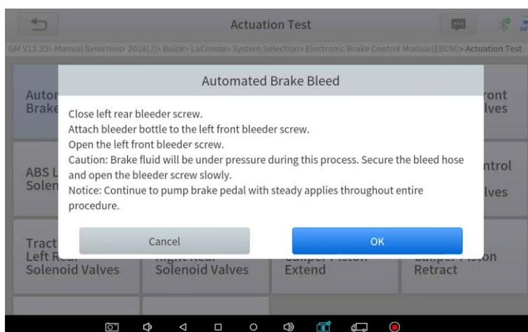
6. Repeat the operation 3 times to complete the bleed procedure for the left front wheel, right front wheel and right rear wheel in turn.
