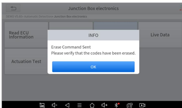
Some troubles are immediately detected by the ECU with the key in the run position and without the engine running. Other troubles are not detected until very specific test conditions are met such as engine coolant temperature within a range, speed within a range for a duration of time, throttle percentage within a range, etc.
